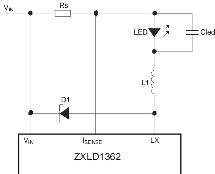
A value of  $1\mu F$  will reduce the supply ripple current by a factor three (approx.). Proportionally lower ripple can be achieved with higher capacitor values. Note that the capacitor will not affect operating frequency or efficiency, but it will increase start-up delay, by reducing the rate of rise of LED voltage.
