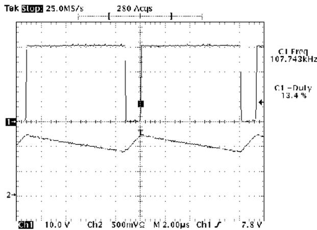
**Actual operating waveforms [ $V_{IN}=60V$ ,  $R_S=0.1V$ ,  $L=100\mu H$ ]**
