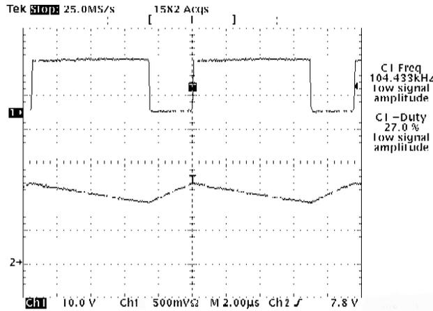
**Actual operating waveforms [ $V_{IN}=30V$ ,  $R_S=0.1V$ ,  $L=100\mu H$ ]**
