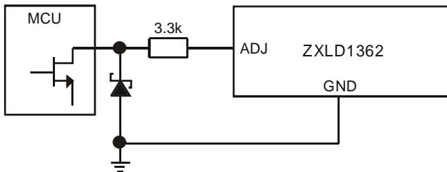
If the NMOS transistor within the microcontroller has high Gate / Drain capacitance, this arrangement can inject a negative spike into ADJ input of the 1362 and cause erratic operation but the addition of a Schottky clamp diode (cathode to ADJ) to ground and inclusion of a series resistor (3.3k) will prevent this. See the section on PWM dimming for more details of the various modes of control using high frequency and low frequency PWM signals.
